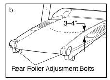
belt centered. Plug in the power cord, insert the key and run the treadmill for a few minutes. Repeat until the walking belt is properly tightened.
